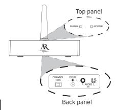
**SIGNAL** indicator lights green when the audio is present and the transmitter is broadcasting
